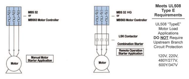
The MBS32 / MBS63 Motor Protectors are an "excellent" choice for <u>ALL TYPES</u> Protector Applications. They are also UL Listed as for use in Group Motor Installations Typical Group Installations shown below:
